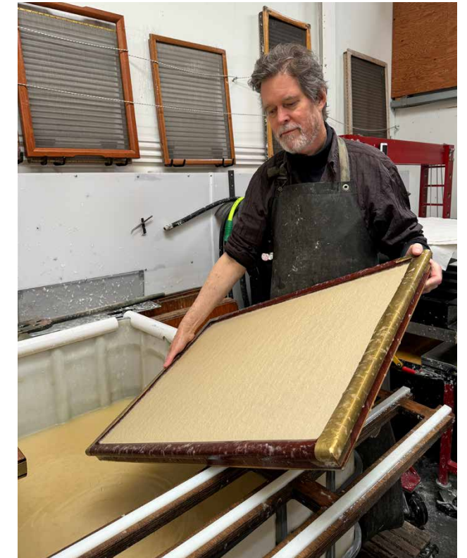
20" x 30" laid paper mould tilted to the bon carron
