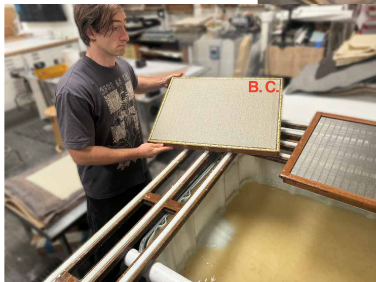
Coucher (Max Thill) takes the mould from the vatman (once the deckle is removed) and then tilts the mould to continue the bon carron draining.
