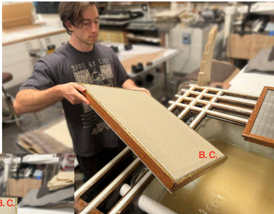
Coucher (Max Thill) takes the mould from the vatman (once the deckle is removed) and then tilts the mould to continue the bon carron draining.
