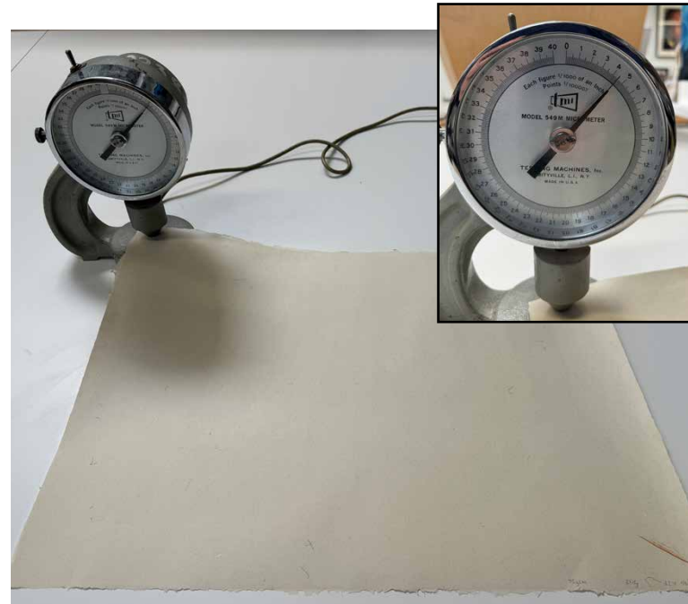
Motorized micrometer measuring the corners in mils (1/1000 of an inch)
