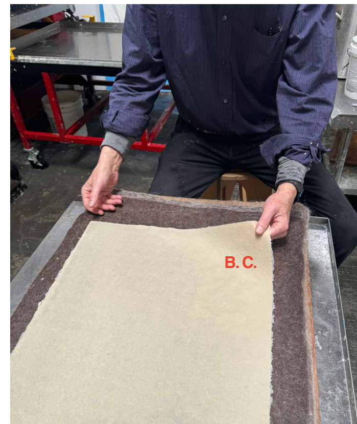
Parting a sheet from a felt lifting from the bon carron corner
