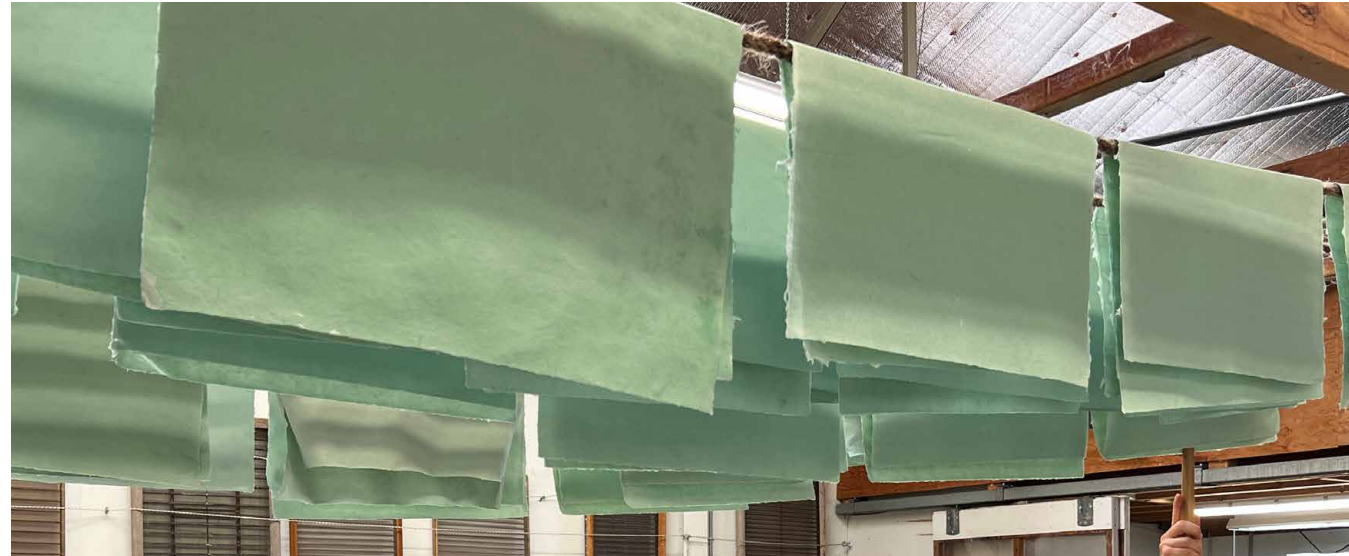
Sheets hung on treble lines to dry (unconstrained and free to cockle and warp)
