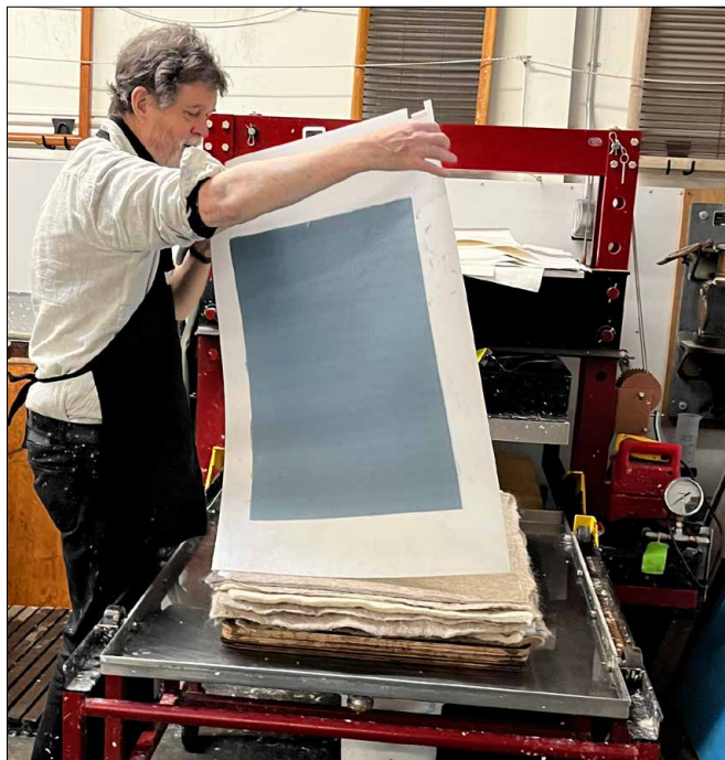
Parting - lifting two sheet at once and hanging to dry
