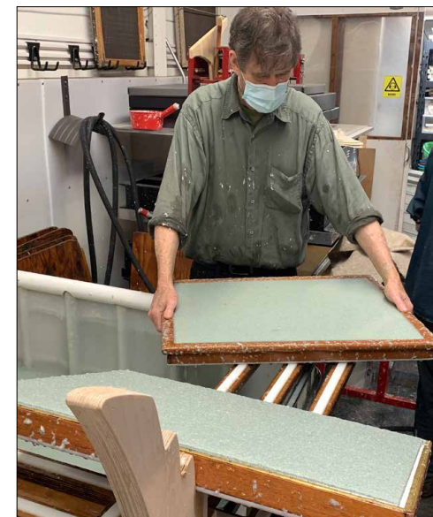
Draining: One sheet draining, leaning of the asp, while a second sheet is formed.
