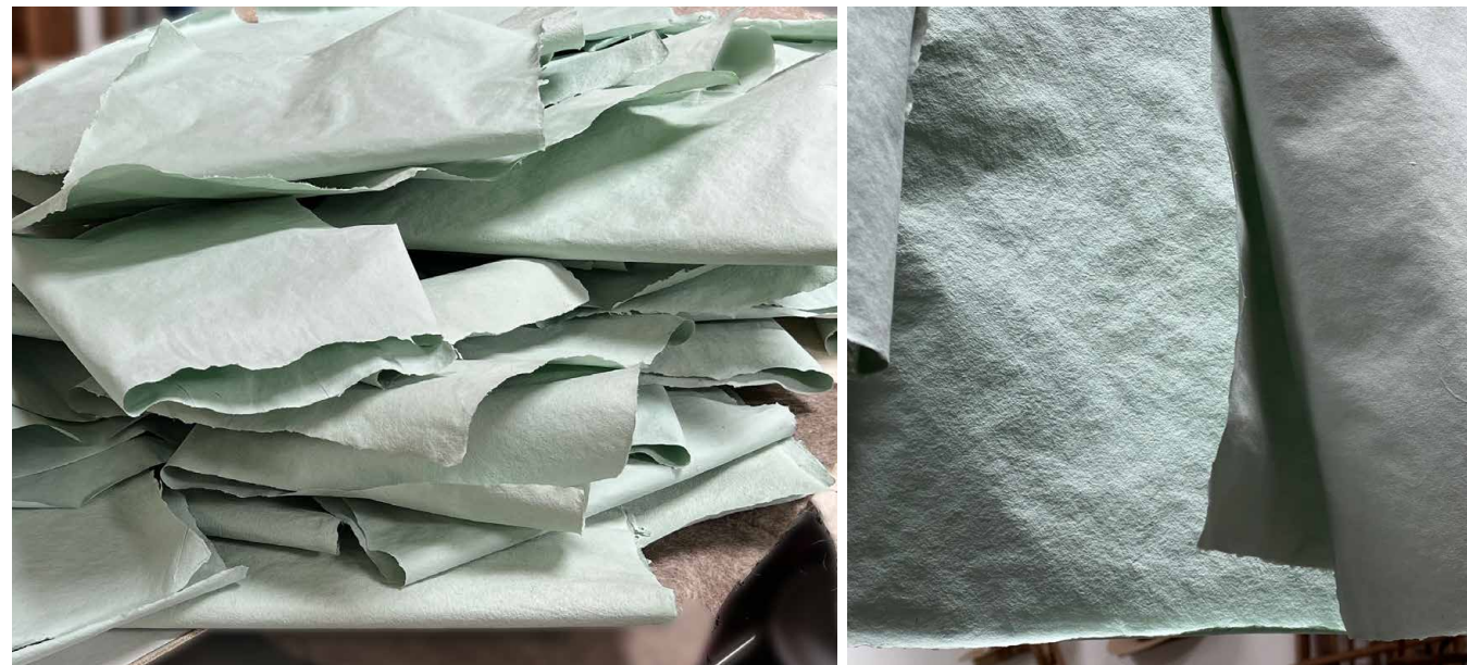
Once dried, the sheets exhibit a beautiful surface texture, but have shrunk and cockled requiring aggressive flattening
