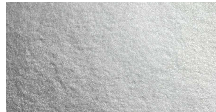
Interfacing that developed a pebbles surface texture
