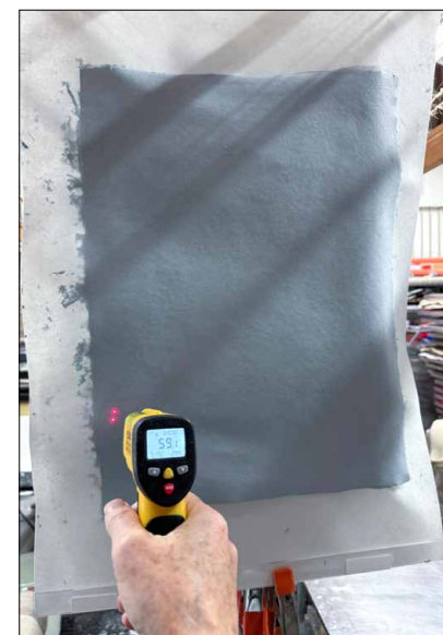
A laser thermometer, is used to determine the paper's state of dryness. Moist surfaces have lower temperatures (indicating evaporation).
