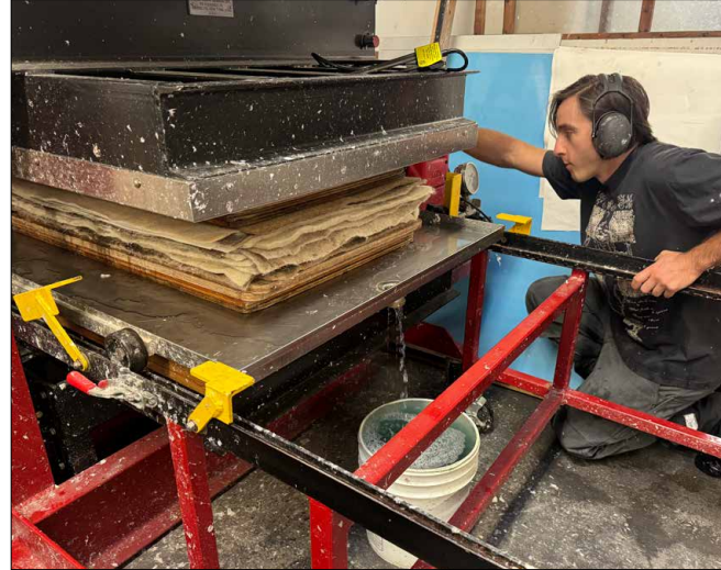
Pressing the post to 50 tons
