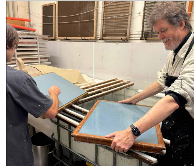
Forming sheets on paired 18 x 24-in moulds (two moulds one deckle)
