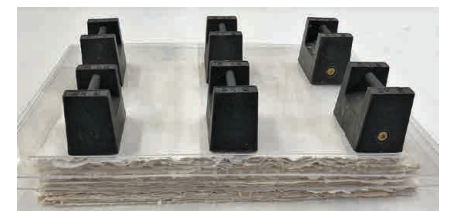
Curing under the pressure of 5kg weights
