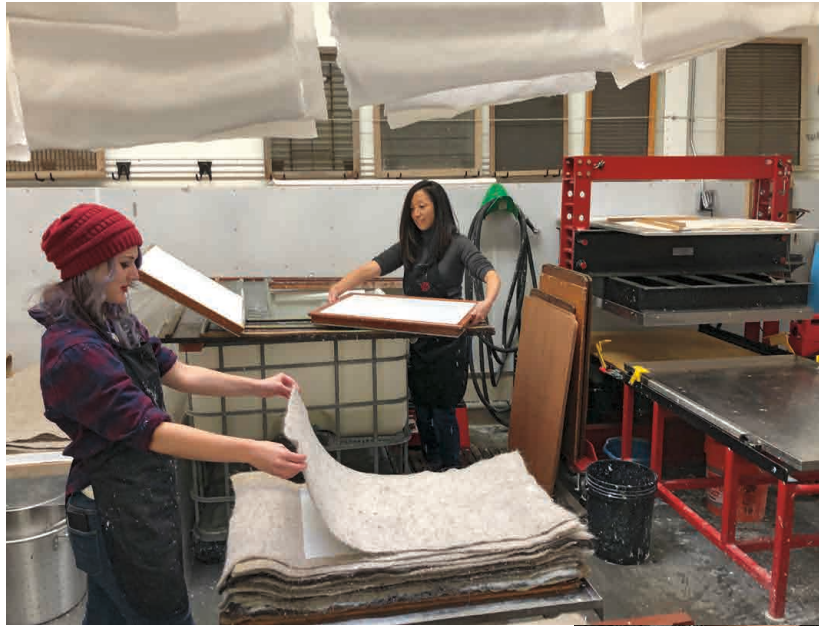
Krista Wright laying felt, Arlene Suda forming
