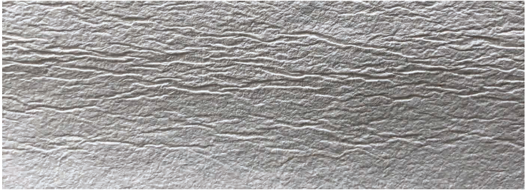
Conversely, the concave texture of this back mark on the verso on the sheet above identifies the wire side.
