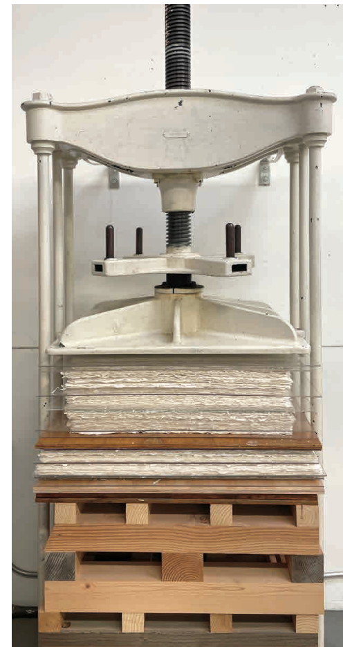
Greater pressure of a standing press used in the final stages of flattening
