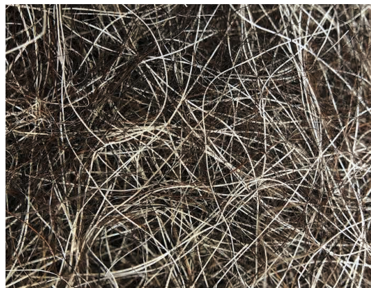
Navajo-Churro wool felt magnified x10
