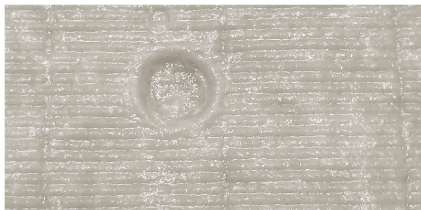
Coucher's drip mark on the wire side of a couched sheet; at right, a similar sheet after drying.
