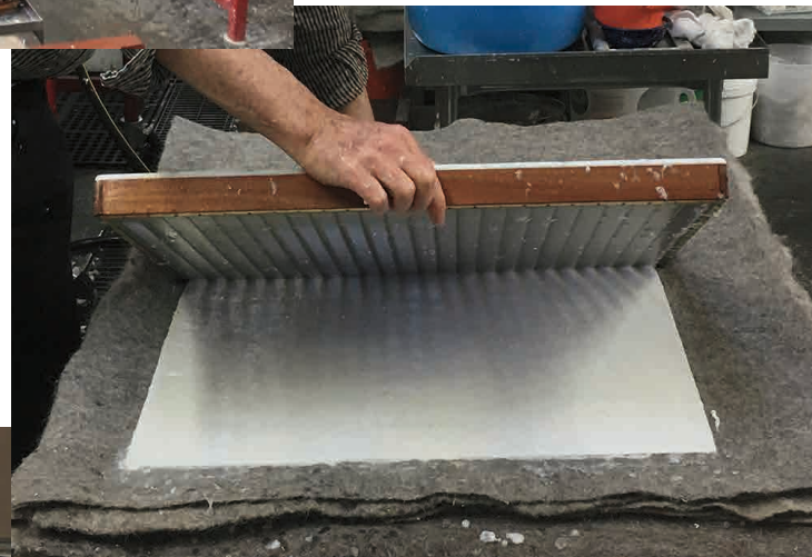
Couching on coarse non-woven Churro felt
