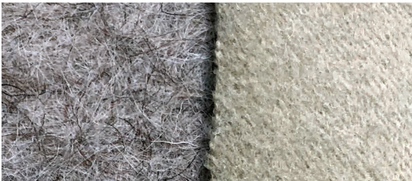
Churro handmade felt at left; an industrial woven and “needled” wool felt at right
