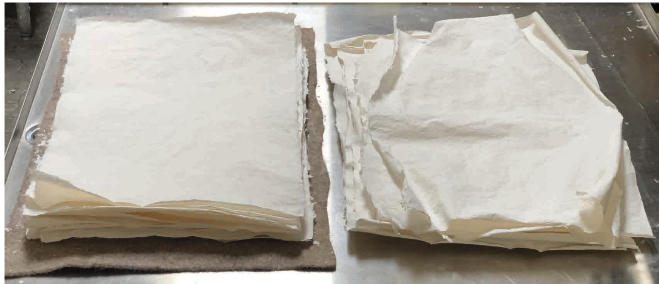
Papers dried individually, unconstrained. Sheets in the left-hand stack were dried on a moist felt; sheets at right were dried on treble lines and flat on taut screen drying rack.
