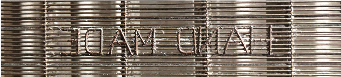
Hand made wire watermark sewn on a laid mould
