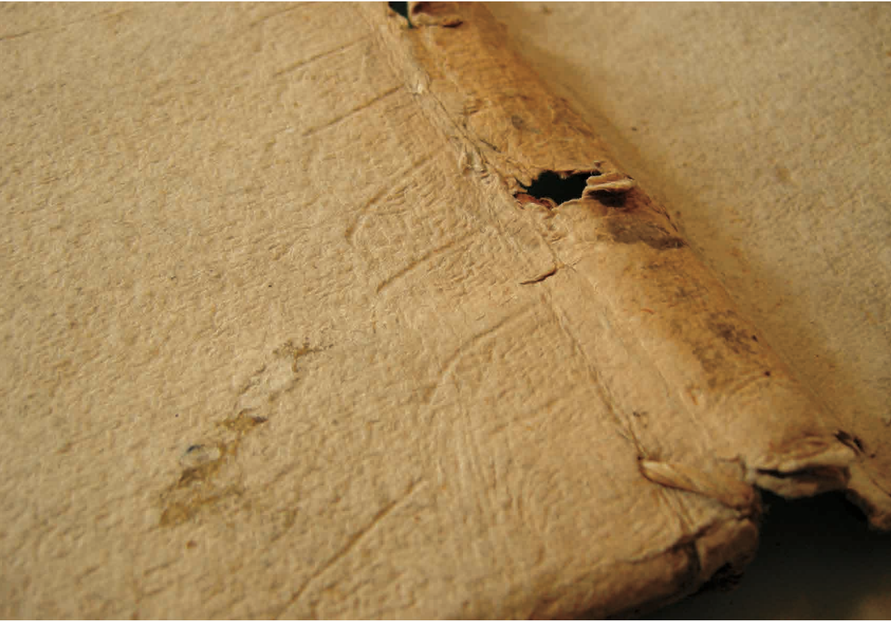
Detail view showing coarse felt hair marks and impressions of stitches used in felt assembly. Photo by Nadine Dumain
