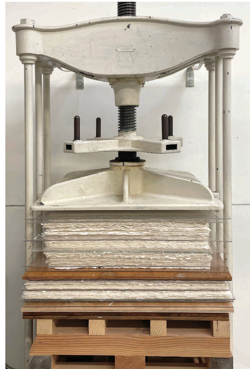
Greater pressure of a standing press used in the final stages of flattening
