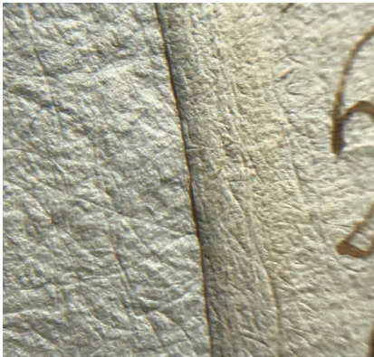
Churro handmade felt on left; an industrial woven and “needled” wool felt on right.
