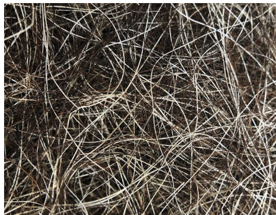
Navajo-Churro wool felt – magnified x10
