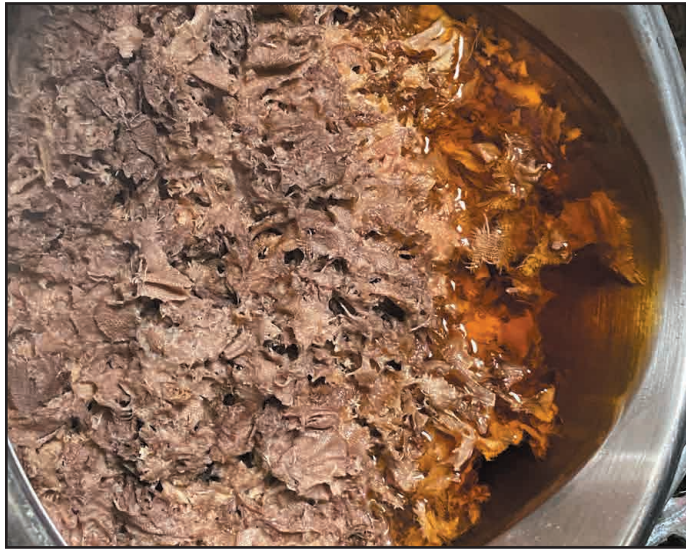
Retted and shredded linen rag in an alkali cook, (soda ash)
