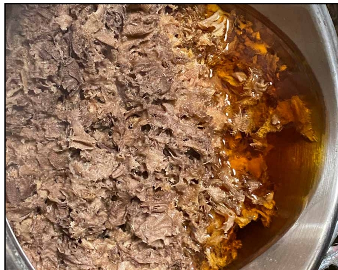
Retted and shredded linen rag in an alkali cook, (soda ash)
