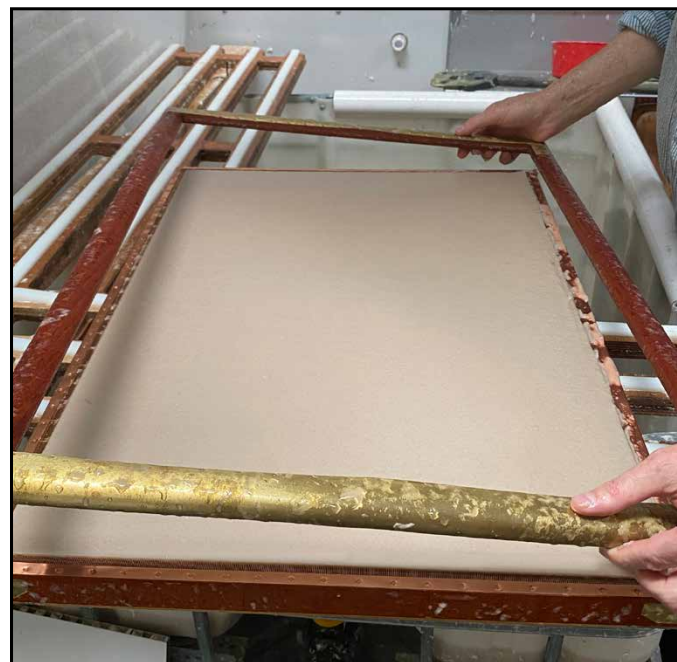
Lifting the deckle – an even sheet edge to edge, corner to corner
