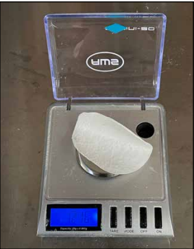
From left to right top to bottom: Beating, Testing Freeness, taking sample from vat, Pouring sample into Arrow Press, Paper Puck at tip of Arrow Press after pressing, The paper puck, Drying puck on inverted iron, weighing puck.
