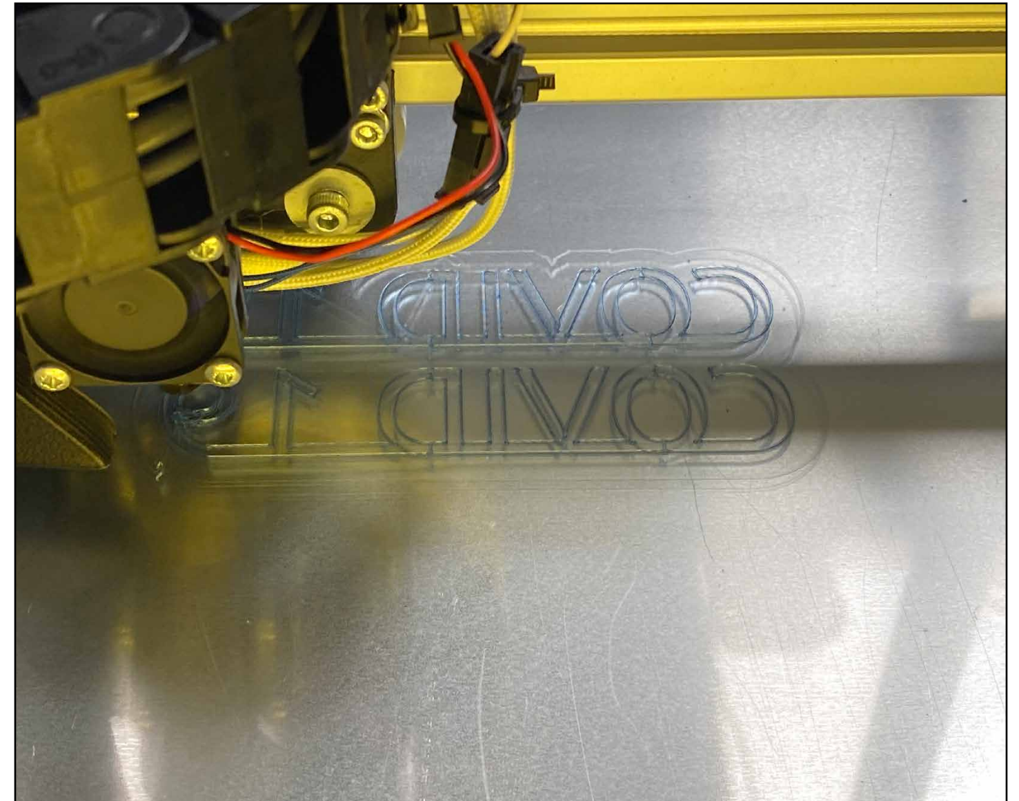
Printing a wire watermark in PLA. The diameter of the extrusion is considered too thin to be successful – not recommended by the manufacturer. “Proceed on an experimental basis.”
