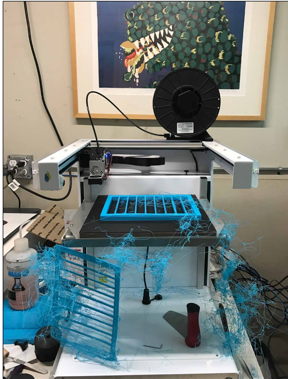
A 3D printed paper mould gone haywire.
