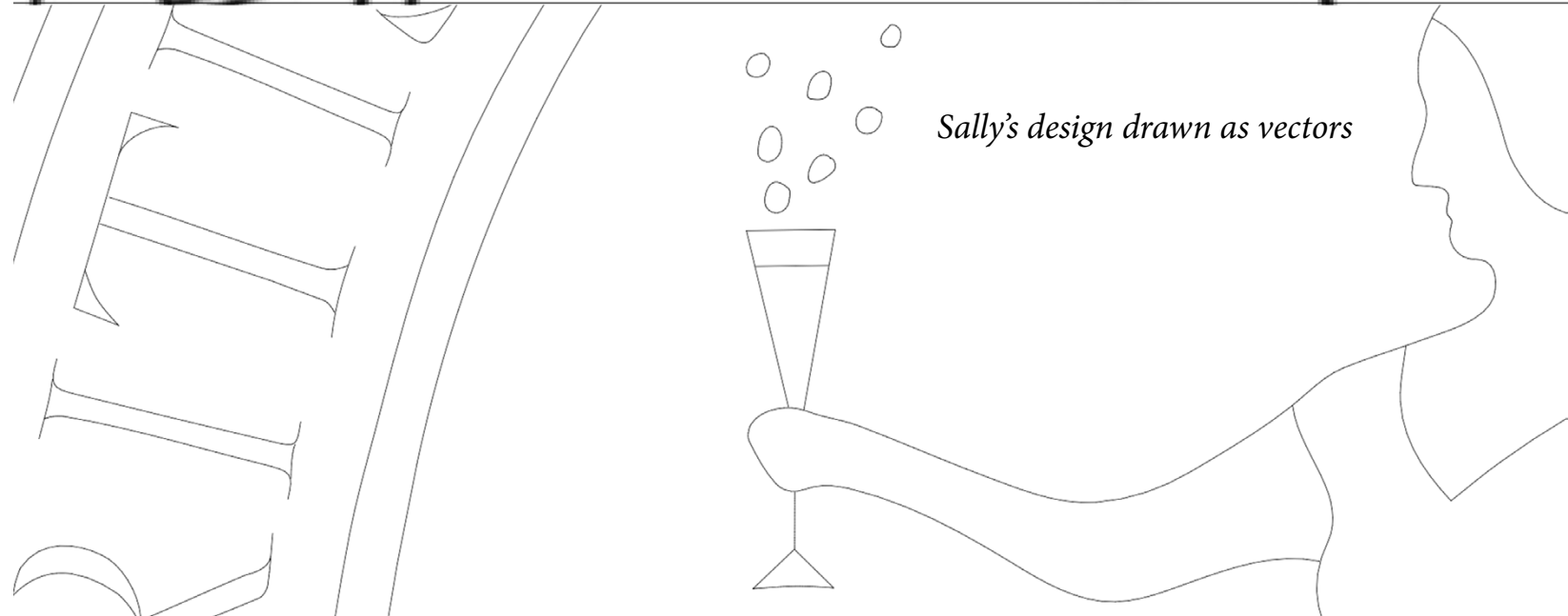
Sally's design outlined with 0.3mm strokes to match the nozzle diameter of the 3D printer. The printer will infill the space between the two lines
