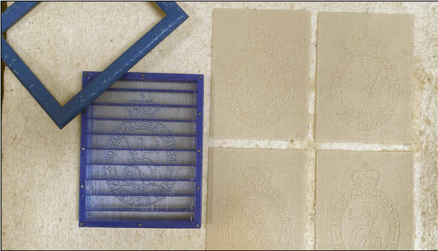
Mould and deckle with watermark infused laid screen and four couched sheets on Fabrianesi and Apenninica wool felt.
