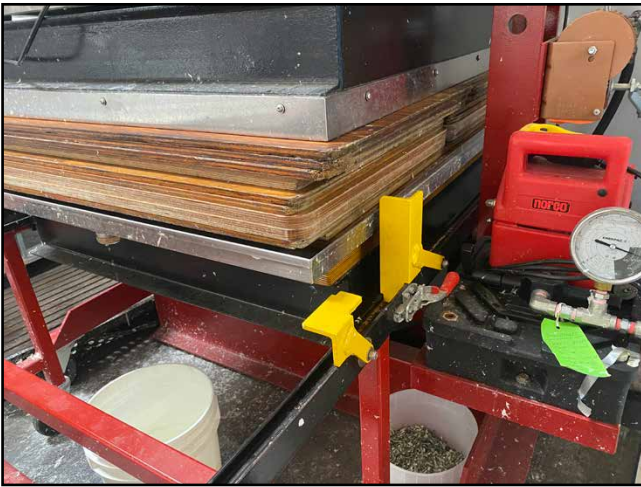
After a few minutes under pressure, we extract the stack of boards and felts from the press and expose our sheets, ready to be air-dried.
