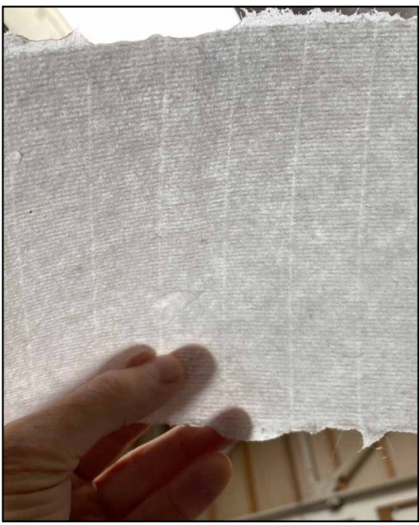
The laid screen covering on the mould gives our Renaissance TP a very nice look-through.
