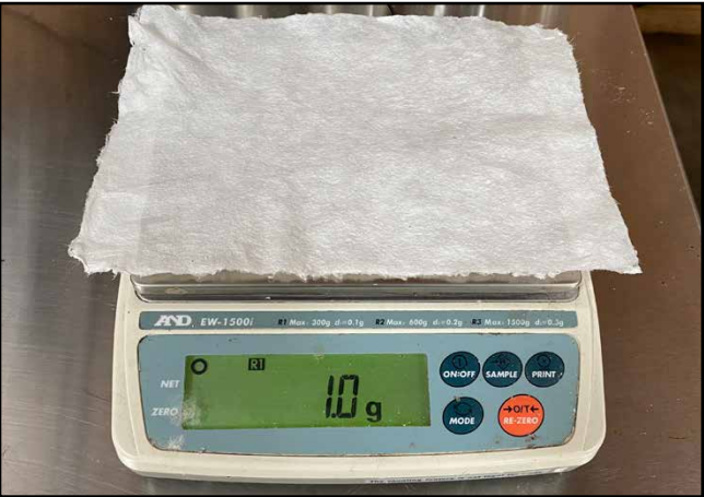
The grams per square meter came in right-on-target, with each sheet weighing 1g, equal to 32.66 g/m2.
