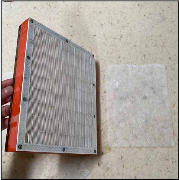
In the spirit of Renaissance paper, I am using a laid paper mould - albeit made from 3D printed plastic.
